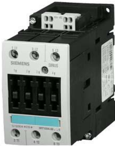
CONTACTOR, AC-3 22 KW/400 V, DC 24 V, 3-POLE, SIZE S2, CAGE CLAMP
