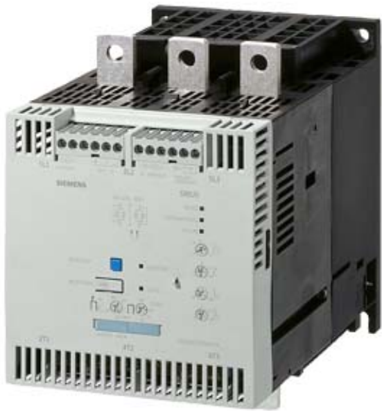
SIRIUS SOFT STARTER, S12, 432 A, 250 KW/400 V, 40 DEG., 200-460 V AC, 230 V AC, SCREW TERMINALS
