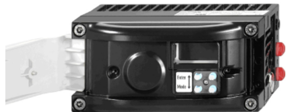
Figure 6: Open TZIDC 200 with a view of the operating panel
