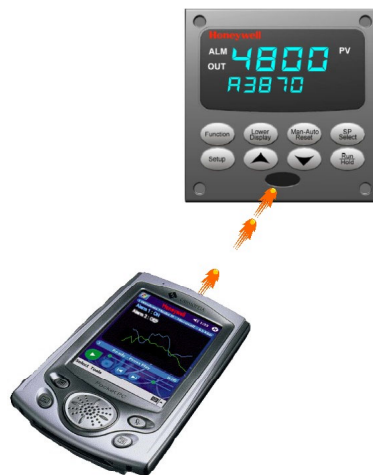
Figure 1-3 Depiction of infrared communications
